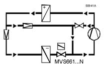
Typical control range 10...100 %. The capacity controller ensures that the compressor is adequately cooled, making it unnecessary to set a minimum stroke in the refrigerant valve.
