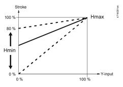
In the case of the suction throttle valve, it is essential that a minimum stroke limit be maintained to ensure compressor cooling and efficient oil return. This can be achieved with a reinjection valve, a bypass line across the valve, or a guaranteed minimum opening of the valve. The minimum stroke can be defined via the controller and control signal Y, or it can be set directly with potentiometer Rv.
